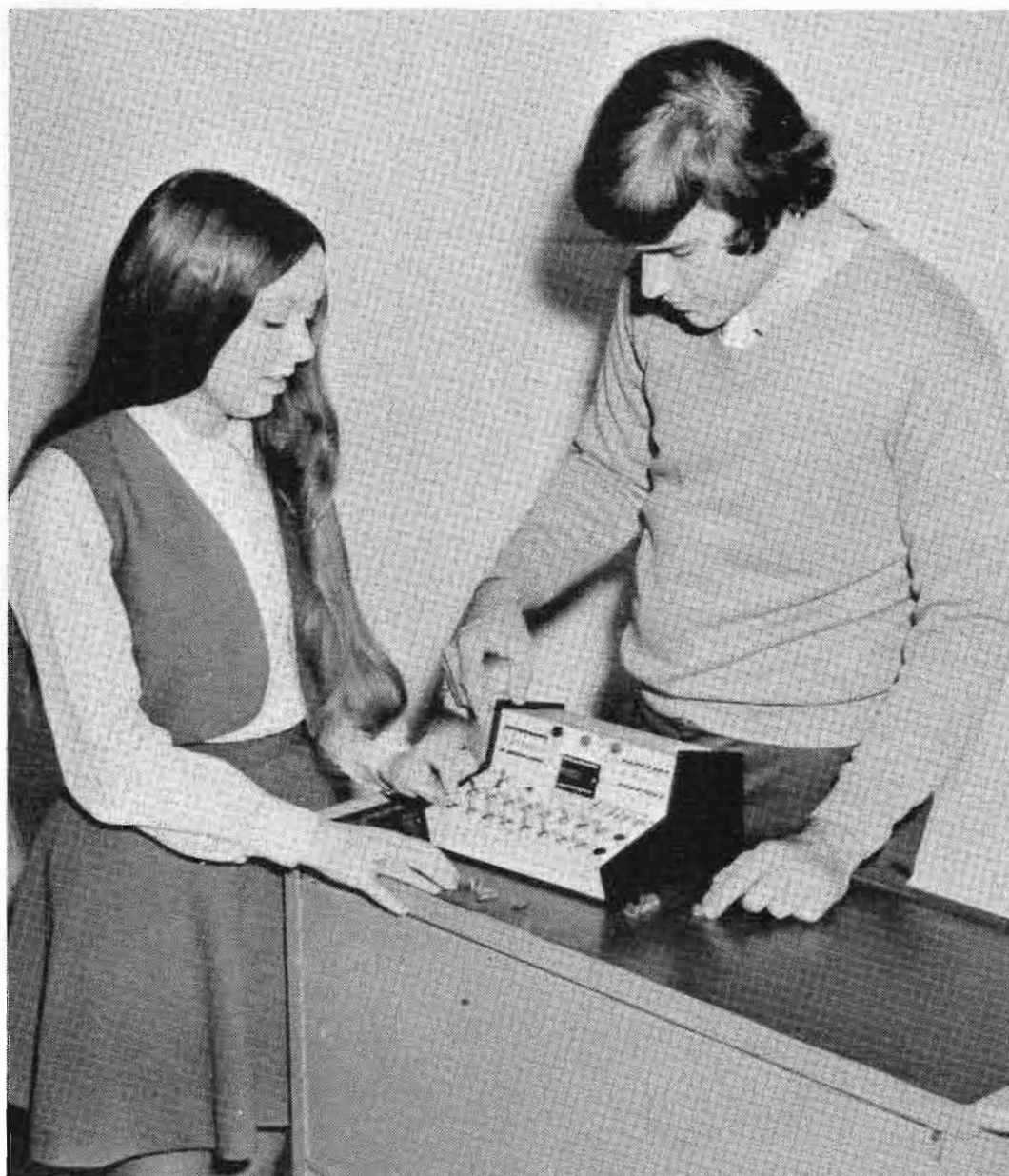
Fig. 3 With the tester completed, Randy fires up the unit by testing a SN7401. Can you test yours?
